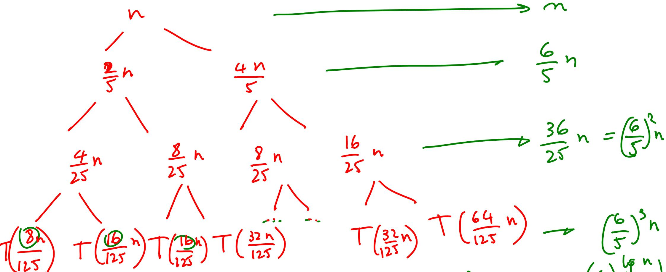
$$T(n) = \Theta\left(n + \frac{6}{5}n + \left(\frac{6}{5}\right)^2 n + \left(\frac{6}{5}\right)^3 n + \dots + \left(\frac{6}{5}\right)^{lg n} n\right)$$
